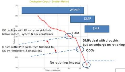
Long run historical data used to determine WR System DO for different RPs and LoS
