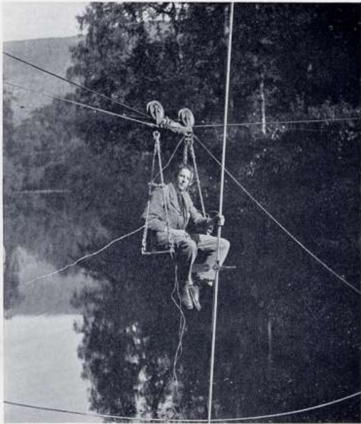
5. Gauging with current-meter from the bosun's chair: Invergarry, 1913
